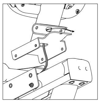
Figure 6: Heart rate sensor cable routing
